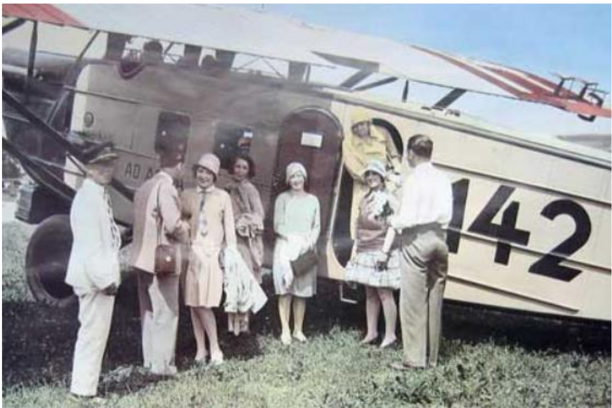
Dornier Merkur CH-142 of the Ad Astra Aero (circa 1927) carried max. 7 passengers with 150 km / h
